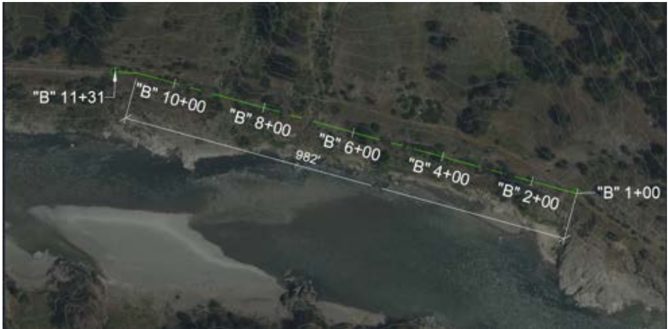
Figure 84: Alignment Alternative “B” – Footbridge Plan View
