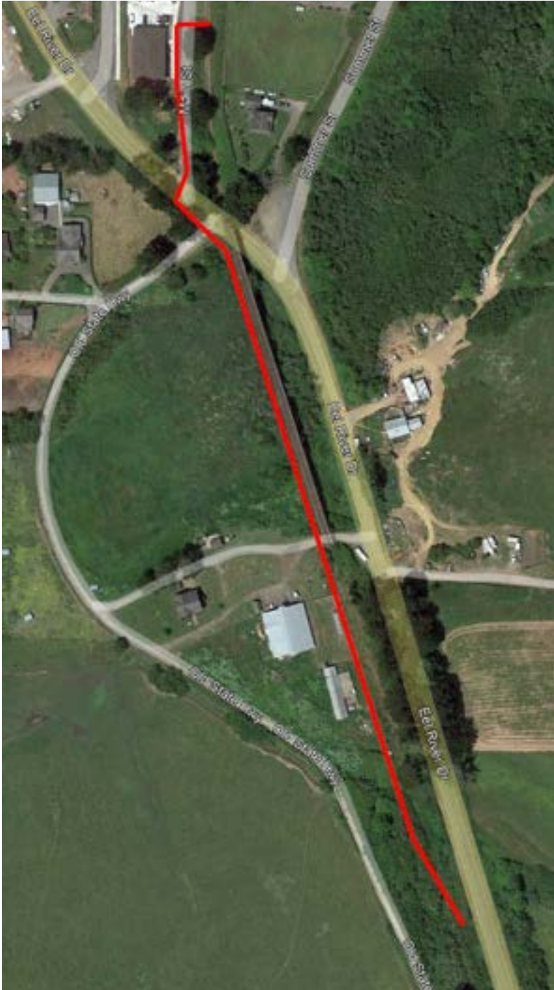
Figure 97: Boardwalk Alignment Plan View
