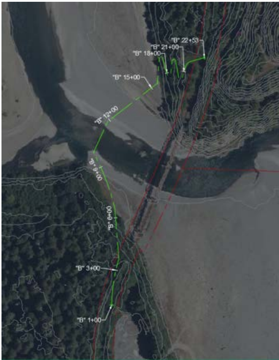
Figure 89: Alignment Alternative “C” – Footbridge Plan View
