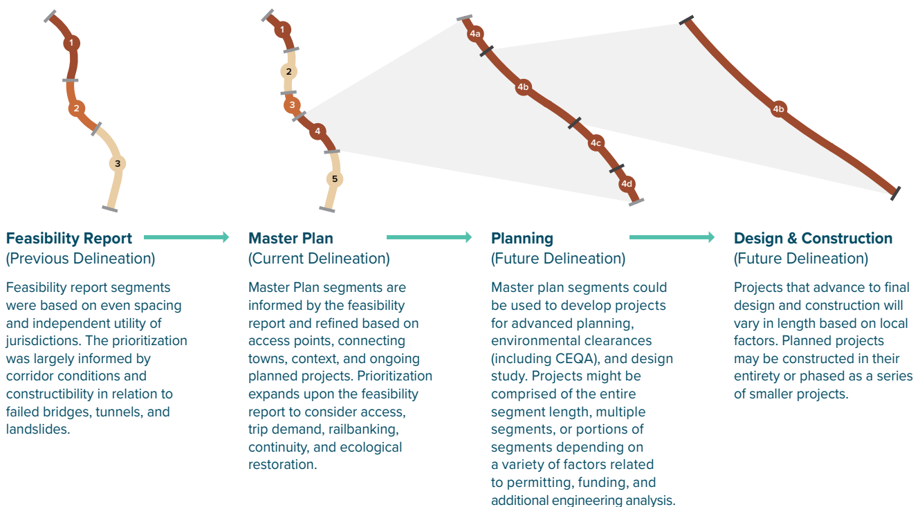
Figure 74: Prioritization flowchart from feasibility report to design and construction of individual projects. The segments referenced in this graphic are for illustrative purposes only and do not align with actual segment or project delineations.
