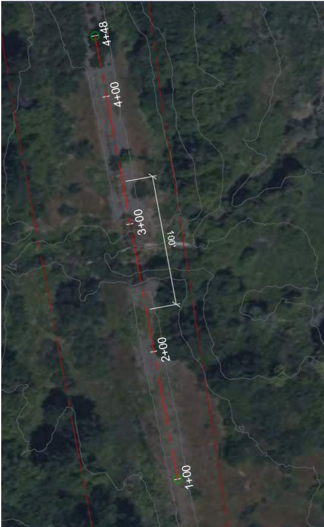
Figure 86: Alignment Alternative - Existing Rail Bed Plan View
