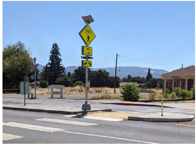
Trail crossings will prioritize safety for all trail users with traffic calming features including pedestrian refuge islands and flashing beacons.
