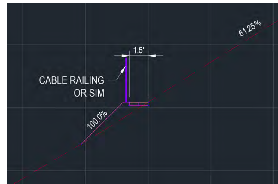
Traverse Alt 2: 1.5' wide built pathway with cable railing or similar.
